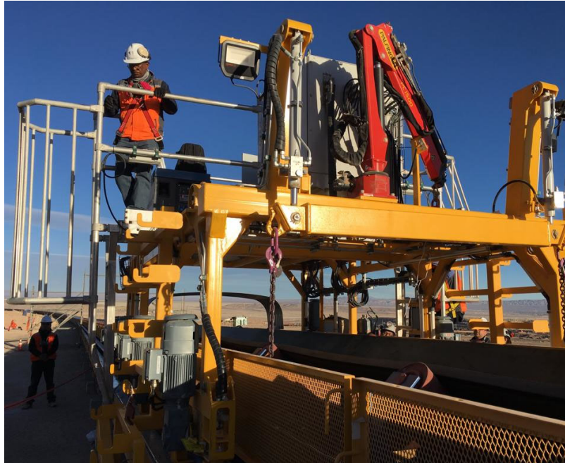
Image 11: TAKRAF maintenance vehicle for safely lifting the belt and replacing the idlers
